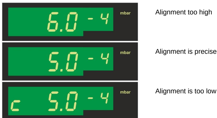
Figure 20 – Zero alignment for the THERMOVAC gauge head
