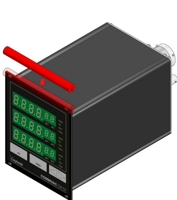
Figure 5 – Preparing the top side of the instrument for utilisation as a benchtop unit
