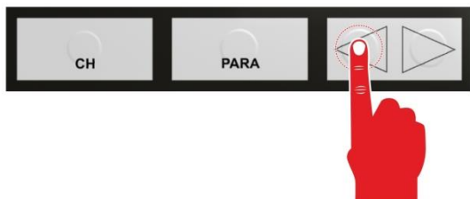
Figure 16 – Operating the pushbutton DOWN
