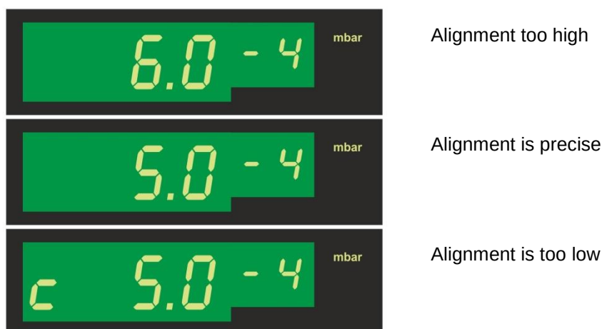
Figure 18 – Zero alignment for the THERMOVAC gauge head
